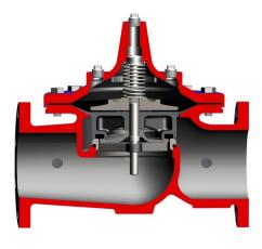
The CLA-VAL Model 100-06S Seawater Service Hytrol Valve is a hydraulically operated, diaphragm actuated, globe or angle pattern valve. It consists of three major components: body, diaphragm assembly, and cover. The diaphragm assembly is the only moving part.
